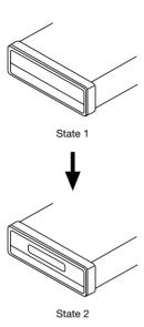
Press o (power) button to turn on the unit. Then press o (eject) button, the panel will turn down to horizontal position (see State 3).
